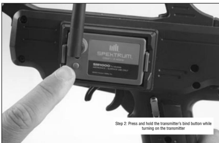
It is necessary to bind the handheld unit to the transmitter. Binding teaches the handheld unit the specific code of the transmitter and when bound, the handheld unit will only listen to information coming from the receiver(s) that are bound to that transmitter. To bind the handheld unit:
