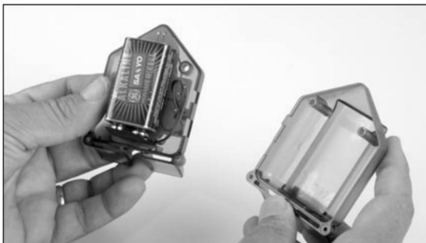
Use 3/32" and 5/64" hex wrenches to unscrew the case and install the 9-volt battery as shown. Reinstall the case, being careful not to over-tighten the screws.
