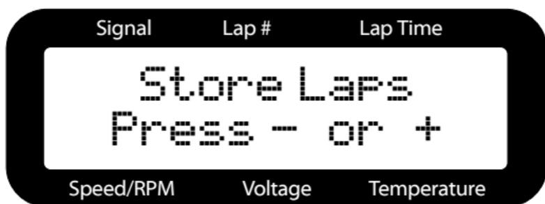
During a run, current lap information is stored in the telemetry module. (Not in the handheld unit). This information is then displayed on the handheld unit. To reset the lap information, it is necessary to turn the receiver off then on. This will reset the lap information and the screen will display 0 laps at 0:00.00 seconds. Previous laps will remain in memory of the handheld unit until it is power cycled.
