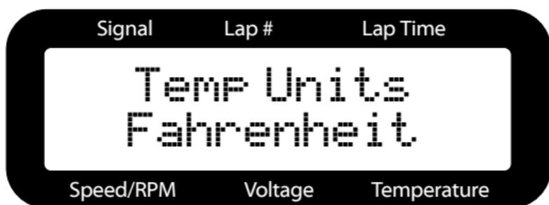
The Temperature Units screen allows you to select between Fahrenheit or Celsius. To access the Temperature Units screen press the  $\uparrow$  or  $\downarrow$  button until **Temp Units** appears on the screen. Pressing the + or – button will change the units from Celsius to Fahrenheit.
