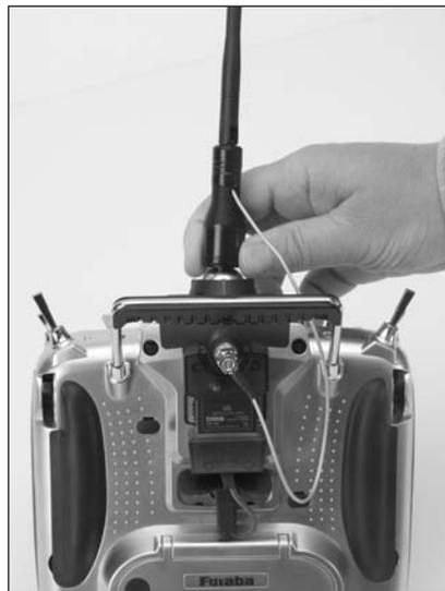
Place the transmitter in PPM mode. This is done in the modulation menu in your transmitter's programming. See your Futaba MZ radio manual for specific details if necessary.
