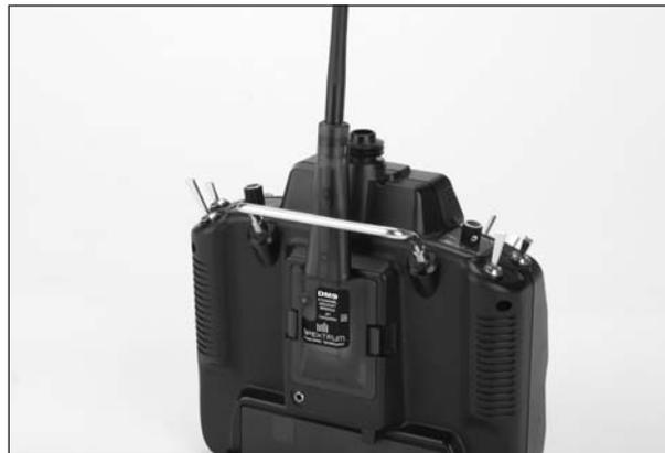
2. Turn on your transmitter. The LED on the back of the module should come on after a few seconds. If not check to be sure the transmitter is in PPM modulation mode (Step 3 in preparing the transmitter above).
