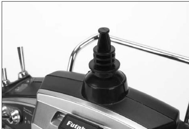
Antenna Adapter installed
