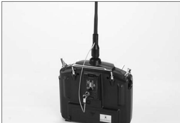
5. Turn on your transmitter. The LED on the back of the module should come on after a few seconds. If not check to be sure the transmitter is in PPM modulation mode (Step 3 in preparing the transmitter above).
