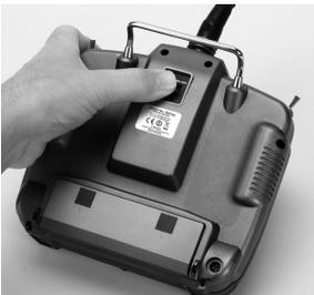
4. Follow the procedures of your specific transmitter to enter Bind Mode, the system will connect within a few seconds. Once connected, the LED on the receiver will go solid indicating the system is connected.
