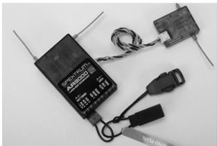
**Note:** To bind an aircraft with an electronic speed controller that powers the receiver through the throttle channel (ESC/BEC), insert the bind plug into the BATT/BIND port in the receiver and the throttle lead into the throttle (THRO) port. Proceed to Step #2.
