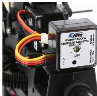
LED off or flashing = Do not fly
