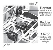
the left, the gyro should react with right aileron. If the gyro output direction is incorrect, use the reversing switch on the gyro to reverse the gyro output.
