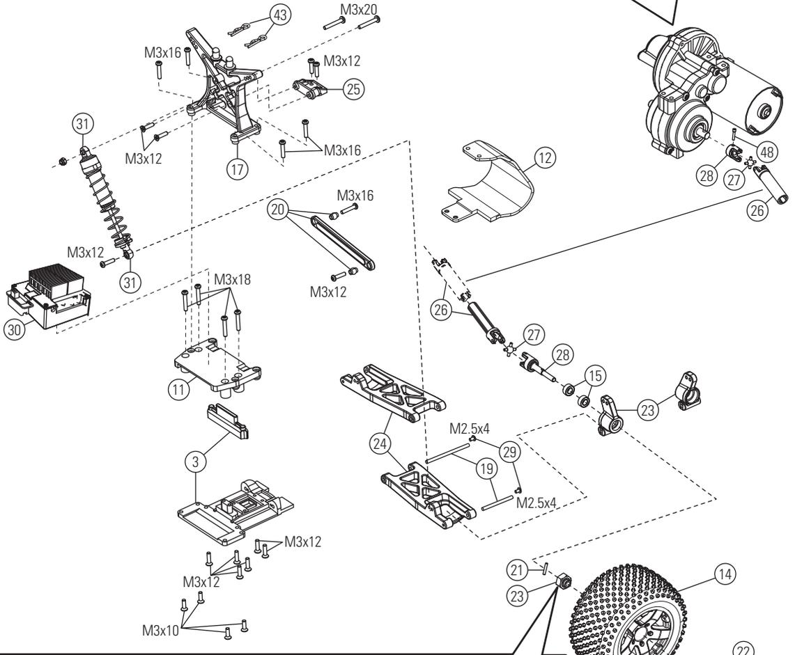
When installing the wheel, make sure the drive hex is aligned with the drive pin. When the drive hex is removed, the drive pin can fall out of the axle.
