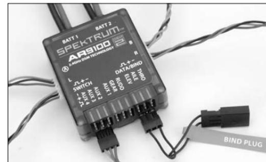
2. Turn on the soft switch. Note that the LEDs on all receivers should be flashing indicating that the receiver is ready to bind.
