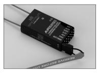
2. Power the receiver through any other port. Note that the orange LED on the receiver should be flashing, indicating that the receiver is in bind mode and ready to be bound to the transmitter.
