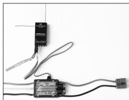
**Note:** To bind an aircraft with an electronic speed controller that powers the receiver through the throttle channel (ESC/BEC), insert the bind plug into the BATT/BIND port in the receiver and the throttle lead into the throttle (THRO) port. Proceed to Step #2.
