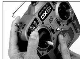
4. Follow the procedures of your specific transmitter to enter Bind Mode, the system will connect within a few seconds. Once connected, the LED on the receiver will go solid indicating the system is connected.
